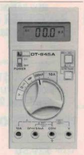
the volts and resistance functions. The 14 mm high display shows the mode of operation, range and polarity of the measurement, along with the value.
