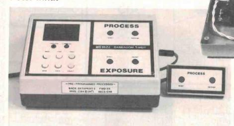
Well, there you are in the darkroom; lights off; photographic paper on the enlarger's baseboard; you switch the enlarger on; you time the exposure with your watch . . . OH NO! — what a time for the batteries to go flat; another wasted print. What you need is an exposure timer like the ETI-662d. Not only does it control your enlarger but it also functions as a process timer — that is, it is two timers in one.
