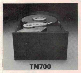
The TM703 and TM705 51/4" high performance Winchester disk drives feature closed-loop positioning. The on-board microprocessor calculates the optimum positioning algorithm, yielding an average access time of 39 milliseconds maximum. Their high capacity makes them ideal for small desktop computers.
